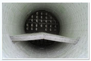
Enclosed flare with an offset wall
